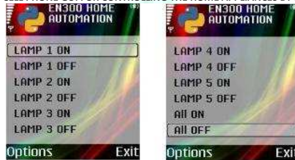
FIGURE 2: CELL PHONE GUI FOR CONTROLLING THE HOME APPLIANCES BY R PIYARE [8]
