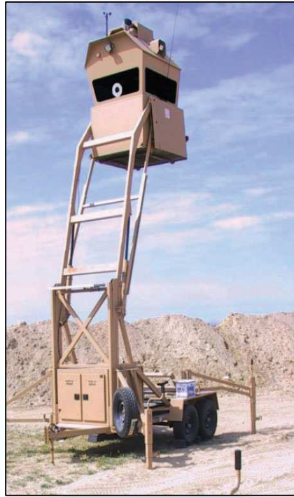
FIGURE 3: MOBILE STATIONARY/SURVEILLANCE TOWERS
