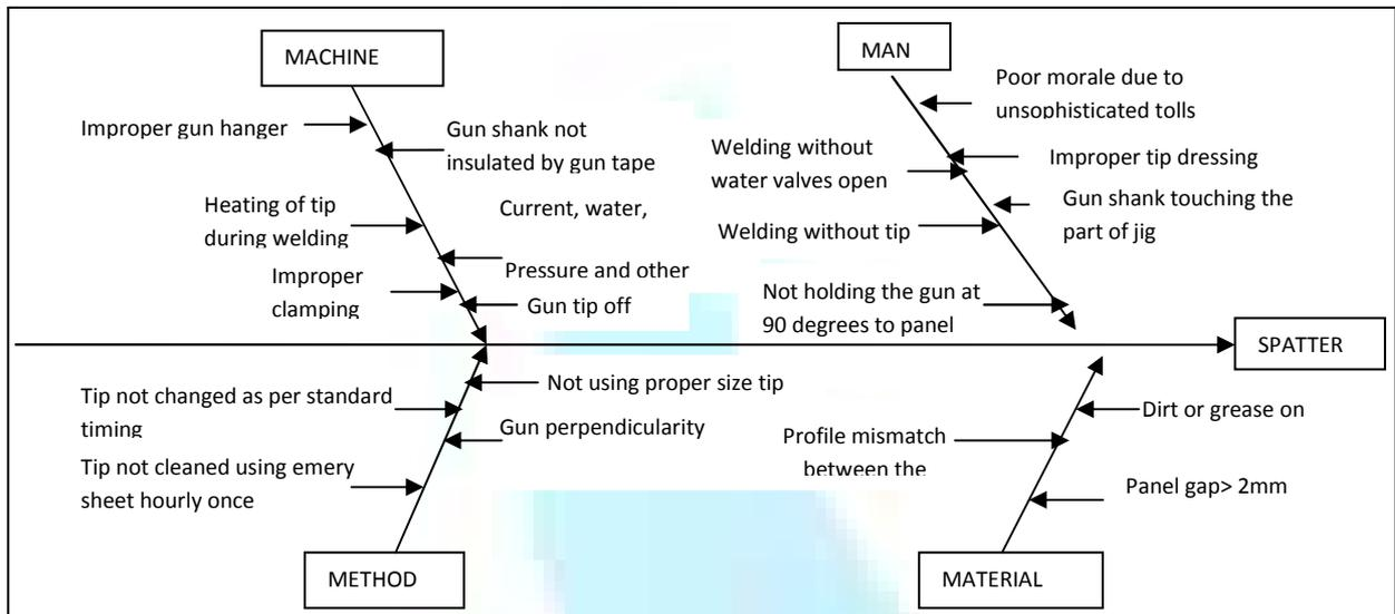
From the above cause and effect diagram, it is analysed that the following factors were the causes for spatter formation;
